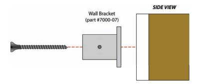
2. Slide the end of the track over the Wall Bracket.
