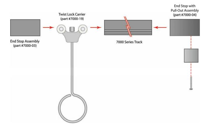
Cut track to length and attach end stops (use End Stops in pairs- one with a pull-out, and one without). Secure track to ceiling (see ceiling mount drawings). Once track is securely mounted, remove pull-out from end stop, insert the I.V. carrier of choice (Twist Lock carrier shown), and reinsert pull-out into the end stop.
