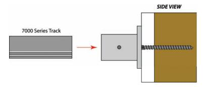
3. Secure track to the Wall Bracket using a two self-tapping screws inserted into the small holes on each side of the Wall Bracket.
